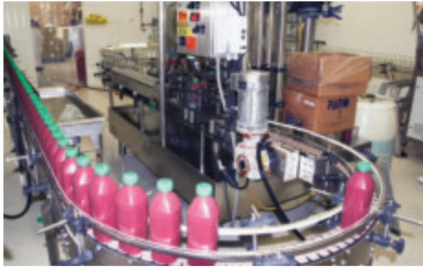
After filling the bottles, a Filler Specialties machine quickly applies the plastic caps on top at speeds of up to 70 bottles per minute.
