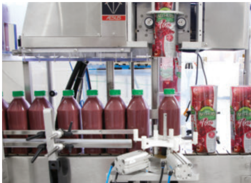
Bottles of fruit smoothies have full-body shrinksleeves applied by an Aesus shrinksleever before moving into a heated shrink tunnel to have the wrap formed around the body.
