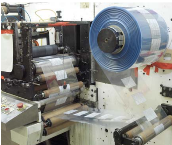
PETG film from Klößner Pentaplast unwinds after a print job concludes on a Chromas LX eight-color flexo press.
