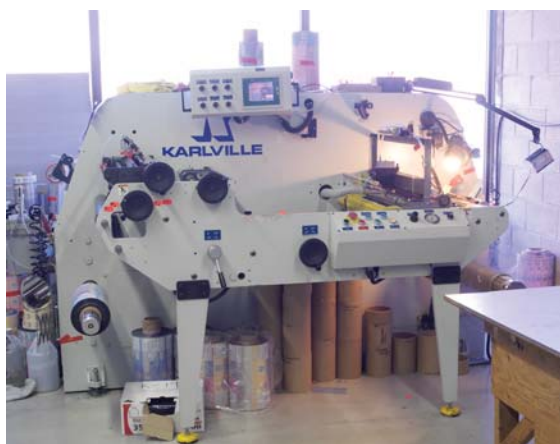
Safety Seal's recently-purchased Hi-Speed seamer from Karlville Development Group features an adjustable forming section.
